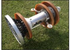
The data-recorder contains all power, processing and recording circuits in a sealed module within the central body of the Caliper-Tool.
