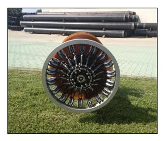
The spider is separate from the cup to eliminate effects from cup wear. As the Caliper-Tool moves through the pipeline, all radial sensor movements are detected and recorded. ID-reductions of 0.4% will be detected.
